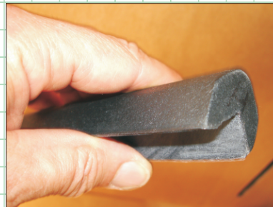
Slim "V" Corner Strips Length: 72" Inside Dimensions: 5/8" x 5/8" Thickness: 5/8"
