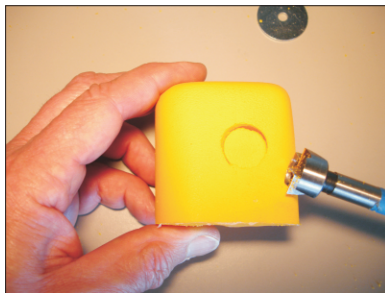
2. Drill with Forstner bit - no more than \frac{1}{2} way
