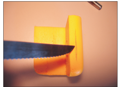
3. Cut slot for washer
